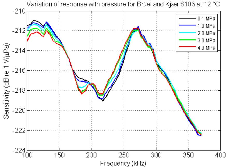
Figure 1. Typical Calibration Curve (OCVR), Conducted as a family of pressure curves
