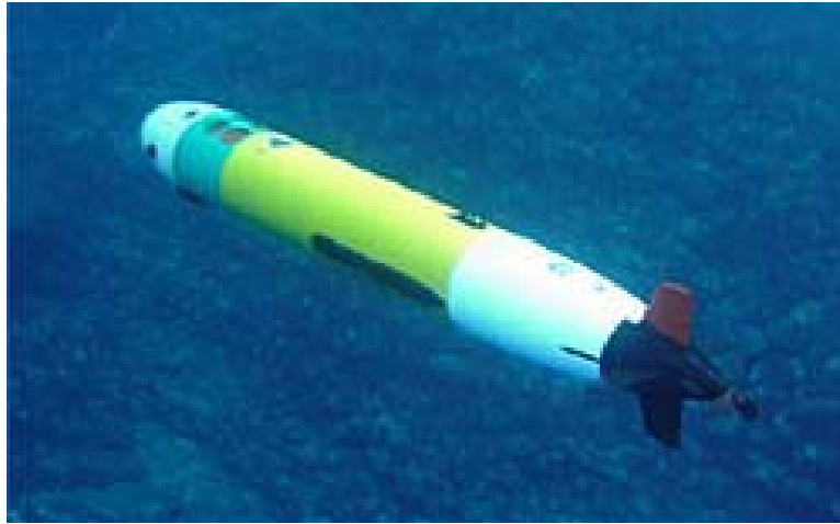
Figure 4.1-7. The Hydroid REMUS, an example of a propeller-driven Autonomous Underwater Vehicle (AUV).
