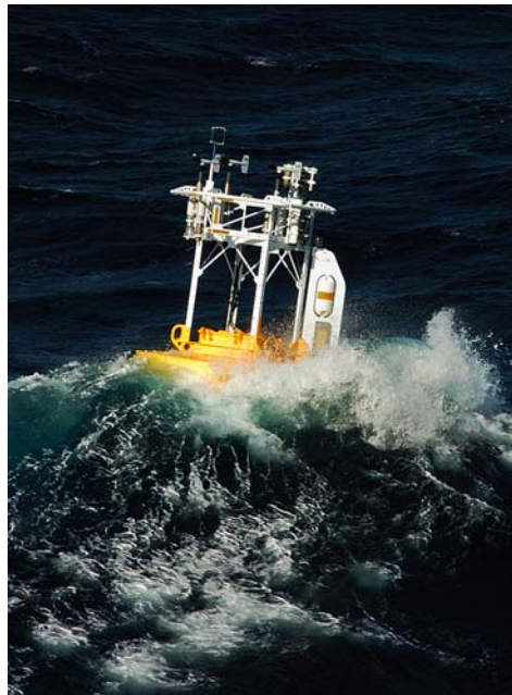
Figure 4.1-3. A 3-m diameter surface buoy on a surface mooring deployed in the Gulf Stream. The buoy carries meteorological sensors, including sonic anemometers for computing turbulent air-sea fluxes.
