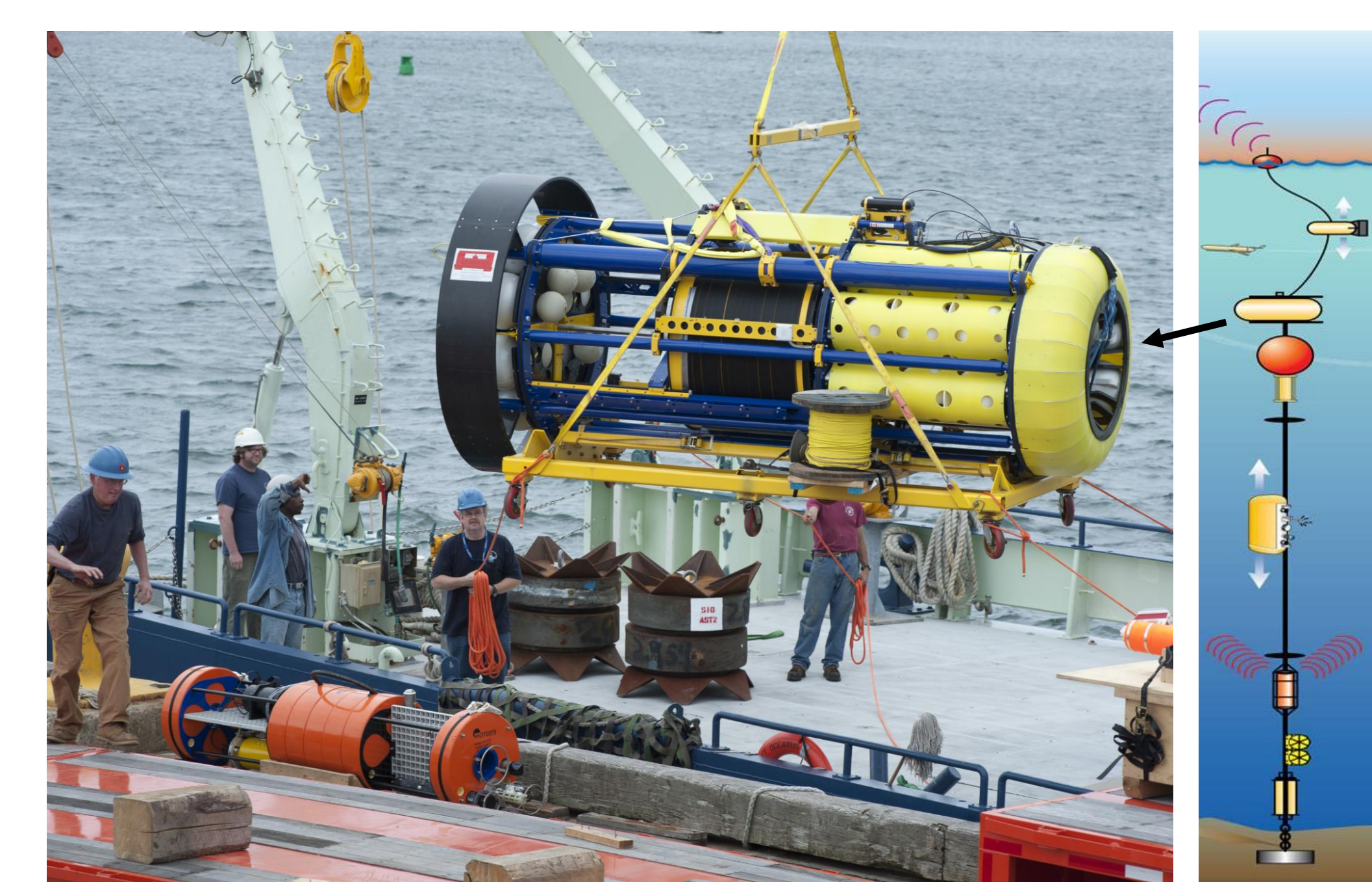
Design test deployment of the Global Hybrid Profiler mooring (left) and conceptual design of the mooring (right). Photo credit: T. Kleindinst, WHOI; graphic credit: WHOI.
