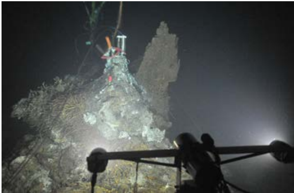
FIGURE 10.1 The RCA cabled digital still camera, redeployed in 2015 by the Canadian ROV ROPOS, lights up the active hydrothermal vent called El Gordo in the interantion District Hydrothermal Filed, located at the summit of Axial Seamount nearly a mile beneath the ocean surface. Credit: UW/NSF-OOI/CSSF.
