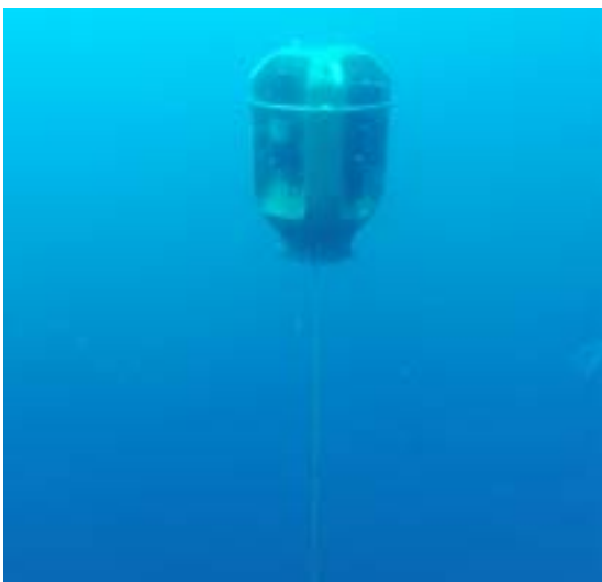
FIGURE 2.17 The Oregon Slope Base Shallow Profiler, engulfed in soft sunlight, rises to 30 m beneath the ocean's surface. It is measuring nutrients, dissolved oxygen, seawater acidity, temperature, chlorophyll, and carbon dioxide concentrations (using the Sunburst SAMI-CO 2 , at left) at high temporal and spatial resolution, controlled from >200 miles onshore through the Internet at the University of Washington. Credit: NSF-OOI/UW/ISS; V15.
