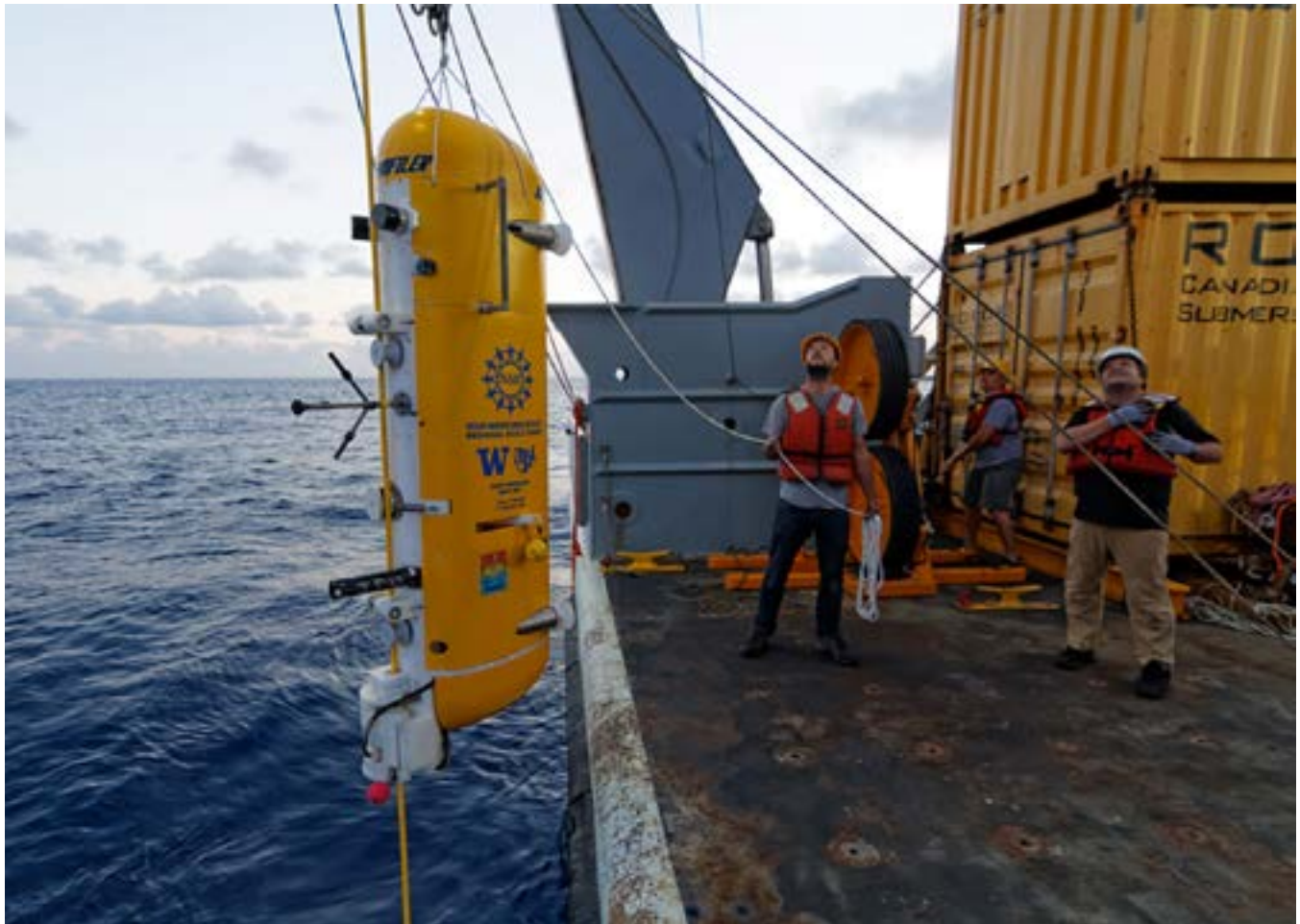
FIGURE A. An RCA instrumented Deep Profiler installed off the fan tail of the R/V Thomas G. Thompson during the 85-day 2014 installation cruise led by Chief Scientist John R Delaney, University of Washington. Credit: M. Elend, University of Washington, V14.
