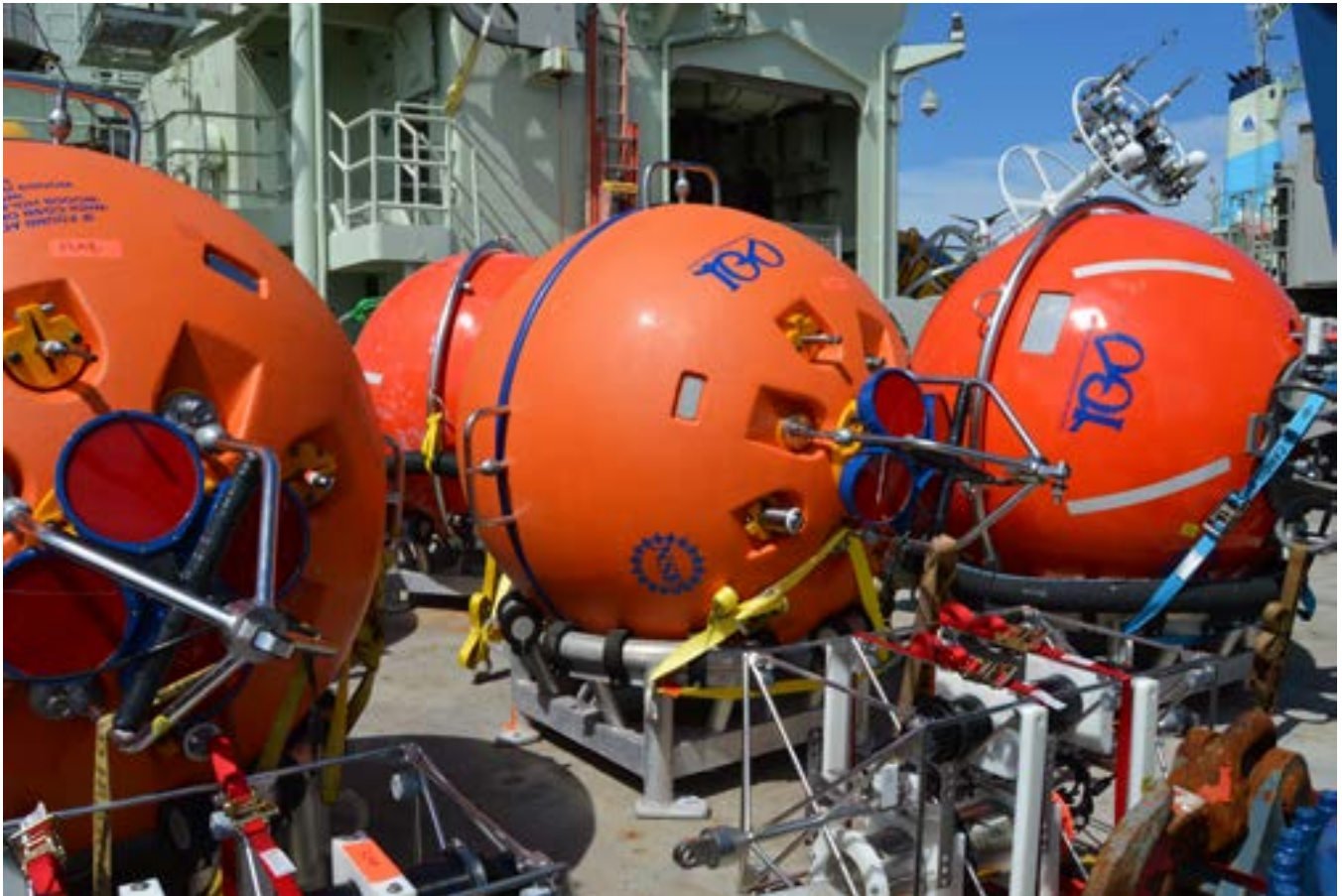
FIGURE 1.3. Sub-surface floating spheres and controllers for two flanking moorings and the Global Profiler await deployment in the Irminger Sea Array. These instruments measure water velocity from the depth of the spheres (500 meters) to the sea surface. Credit: Sheri N. White, Woods Hole Oceanographic Institution
