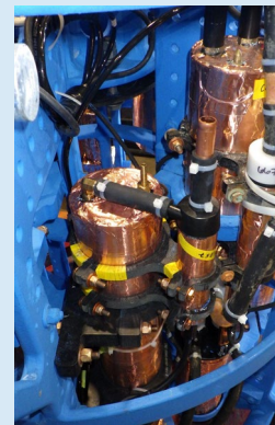
CO 2 -Pro CV mounted on the 7 m platform (Near-Surface Instrument Frame, NSIF) showing intake plumbing and exhaust.
